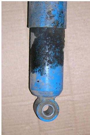
Replaceable leaking shock absorber
