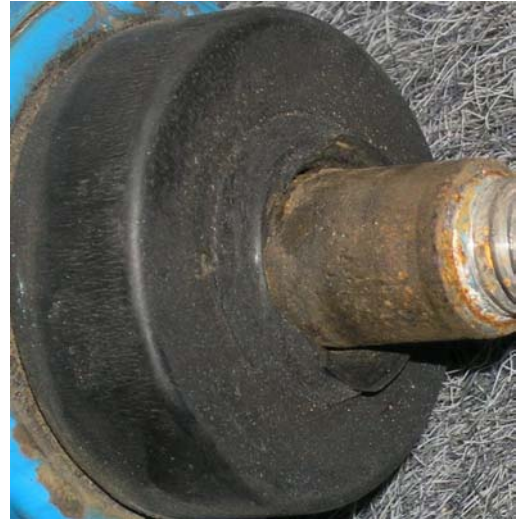
Rubber shoulder premature wear
