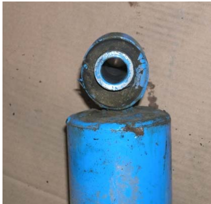
Eye or rubber distortion
