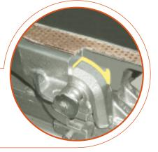
The replaceable lube plate inserts are mechanically-bound to a unique "perforated" plate that provides friction-free performance and extends the life of the lube plate compound. The lube plates fit into cast recesses of the top plate and are secured by studs and locknuts.
