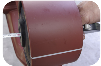
Fig. 16 · Checking the spring center
