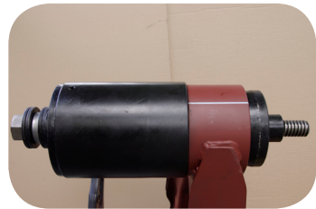
Fig. 6 · Removal tool installation
