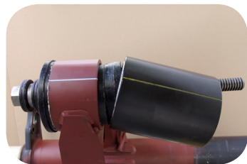
Fig. 15 · Loose receiver tube
