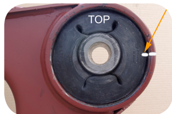
Fig. 4 · Raised bushing position locator
