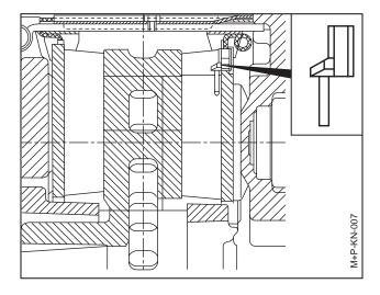
c) Wear Indicator using built-in Potentiometer. This is available either as an on/off version or as a continuous signal version which can be linked to the vehicle's electronic monitoring systems.
