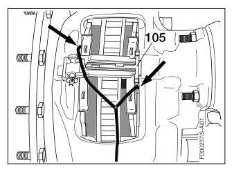
Press Wear Indicator Cable (101) into the locating tabs of the Cable Guide (105) (see arrows A). The short cable end of the Wear Indicator Cable (101) **must not** be secured by locating tabs of the Cable Guide (105).
