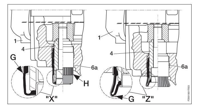
The condition of the Pads can be visually determined without removing the road wheel, by viewing the position of the Caliper (1) against the fixed Guide Pin (4).
