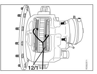
Fit Pad Holder Springs (12/2) onto the Pads (12/1). Pay attention to correct installation of Wear Indicator Cable (101) (see arrows).
