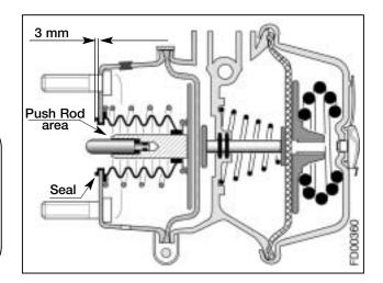
Attach Spring Brake using new Nuts (self-locking EN ISO 10513). In order not to tilt the Spring Brake, screw Nuts step by step alternately with a suitable tool and torque tighten to 180 <sup>+30</sup> Nm.
