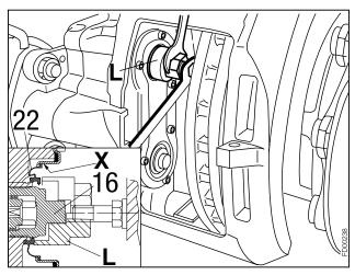
To check the correct fit of the Inner Seal (22), screw out the Threaded Tubes (16) about 4-5 threads by turning the Shear Adapter (61) clockwise. The Inner Seal (22) must not turn.
