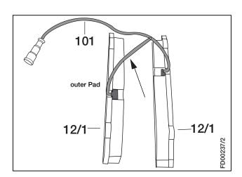
Insert Pads (12/1) into the Pad abutments (see Section 6.2).
