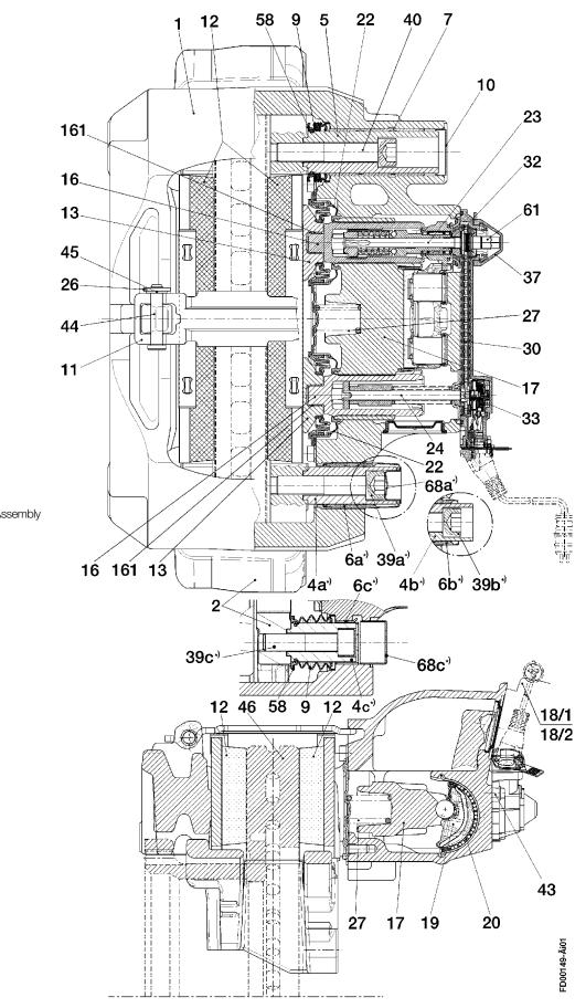
Rubber Bush 6a\*) 6b\*) Rubber Bush 6c\*) Guide Sleeve 7 Brass Bush 9 Inner Boot 10 Cover 11 Pad Retainer Pad (complete) 12 Tappet and Boot Assembly 13 16 Threaded Tube 17 Bridge 18/1 Spring Brake 18/2 Brake Chamber 19 Lever 20 Eccentric Bearing 22 Inner Seal 23 Adjuster Unit 24 Turning Device Spring Clip 26 27 Spring 30 Chain 32 Chain Wheel
