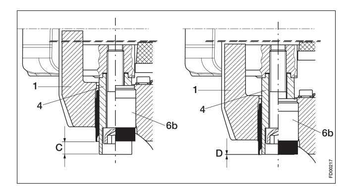
The condition of the Pads can be visually determined without removing the road wheel by viewing the position of the Guide Pin (4) in the Caliper (1).
