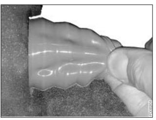
Grease Brass Bush (7) and if installed Guide Sleeve (6c) with **white** grease (Part No. II14525 or II32868).
