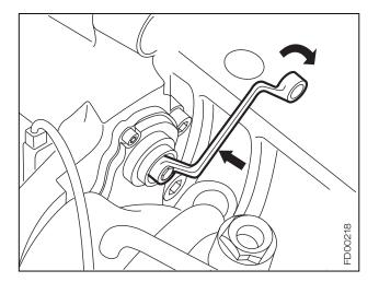
Even if Pads are not being changed, a new Adjuster Cap (37) should be fitted having lightly greased it with **white** grease (available as Part No. II14525 or II32868).
