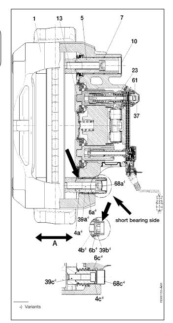
Fasten a magnetic dial-gauge holder to the Carrier (2) on the short bearing side of the Caliper (1) - see also Sketch above.
