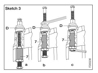
Check contact area of Brass Bush (7) and remove any burrs. Grease Bush (7) with white Grease (Part No. II14525 or II32868).
