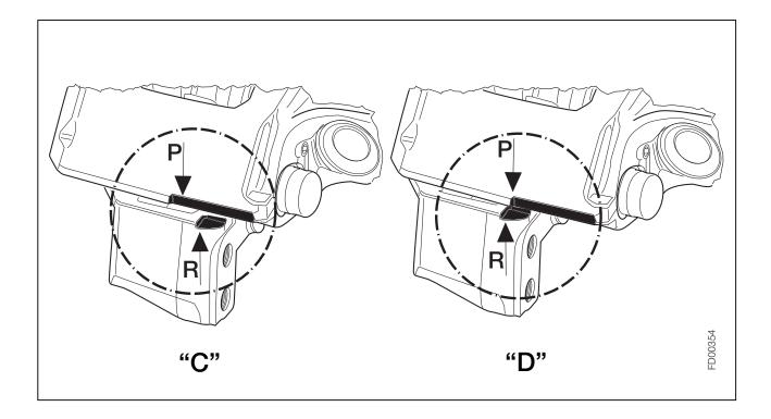
The condition of the Pads can be visually determined without removing the road wheel by viewing the position of the Caliper position (P) against the Carrier marking (R).
