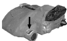
Figure 1: The Type Plate is always on the fixed bearing side
