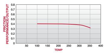
The graph displays the potential change in braking efficiency due to temperature increase. The results are based on the industry recognised SAE J661 test, which provides a measurable frictional output with no mechanical influence.
