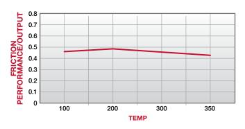
The graph displays the potential change in braking efficiency due to temperature increase. The results are based on the industry recognised SAE J661 test, which provides a measurable frictional output with no mechanical influence.
