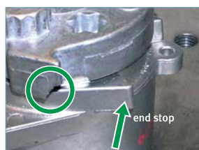
Broken aluminium nose
